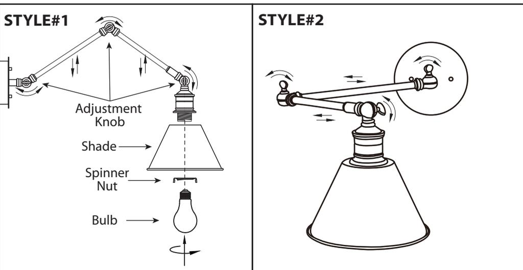
Remove spinner nut from socket. Position shade on lamp and secure with spinner nut. Install specified bulb type and wattage (not included). Adjust the arm of the lamp as desired using the adjustment knob.
