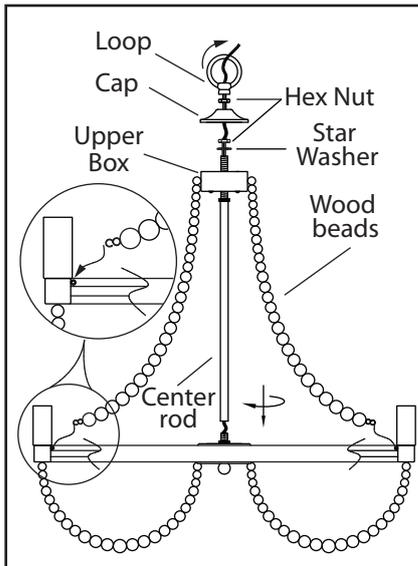
**1.** Screw the center rod to the fixture.
