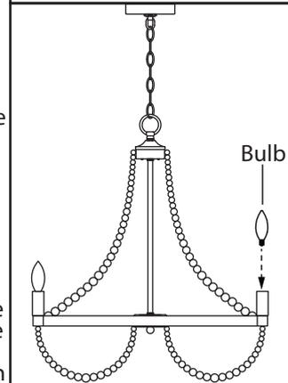
**11.** Slide the canopy up the chain and over the upper connector. Slide the nut up the chain and thread onto the upper connector.
