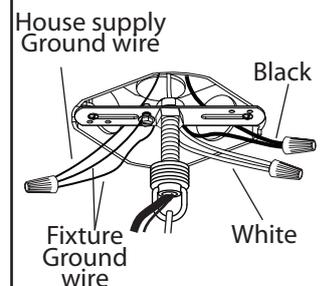
**9.** Connect the ground wires (bare copper or green) from your fixture to the ground wire (bare copper or green) or ground screw in the electrical box. Connect the black wire (or wire marked "SPT-1") from the fixture to the black wire in the electrical box and connect the white wire (or the wire with ribbed side) from the fixture to the white wire in the electrical box.
