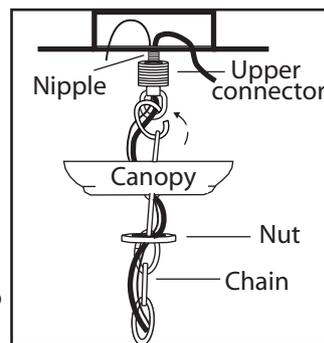
**8.** Loosen the nut on the upper connector and slide it down the chain towards the lower connector. Slide the canopy down the chain towards the lower connector. Feed the wire through nut, canopy, the upper connector and onto the nipple. Tighten the upper connector onto the nipple. Spread the other end of the chain open and fasten to the upper connector. Ensure the opening is closed.
