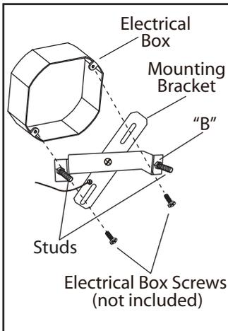
**1.** Loosen "B". Adjust stud to desired length and lock in place with "B".
